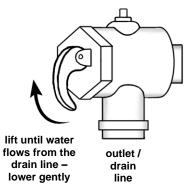
Operate the easing lever on the temperature pressure relief valve and expansion control valve once every six (6) months to clear any deposits and ensure the valve and its drain line are not blocked. It is very important the lever is raised and lowered gently. Refer to "Minor Maintenance Every Six Months" on page 12.
