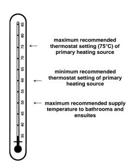
If this storage tank is installed as part of a solar water heater to an in-series continuous flow gas booster, then these AS 3498 and Clause G12 requirements can be satisfied provided the booster is energised, its preset outlet temperature setting is 70°C or higher and a remote temperature controller is not used.
