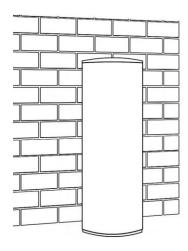
The storage tank is to be installed at ground or floor level and must stand vertically upright on a stable base as acceptable to local authorities. The base of the storage tank is made of corrosion resistant material, and it may be placed directly in contact with the supporting surface. It is not necessary to allow for free air circulation under the base of the storage tank.
