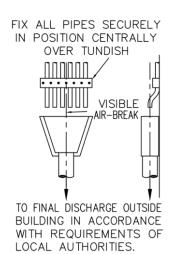
TPR Valve Drain Line Common Discharge Point
