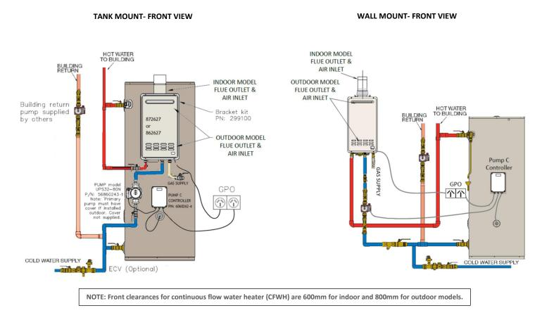
Tankpak 1 models are supplied with tank, pump, controller and an optional tank mounting bracket kit separately.
