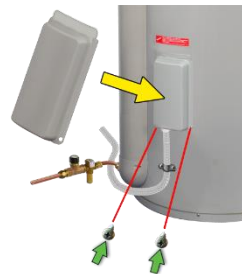
Step 30 refit electrical front cover
