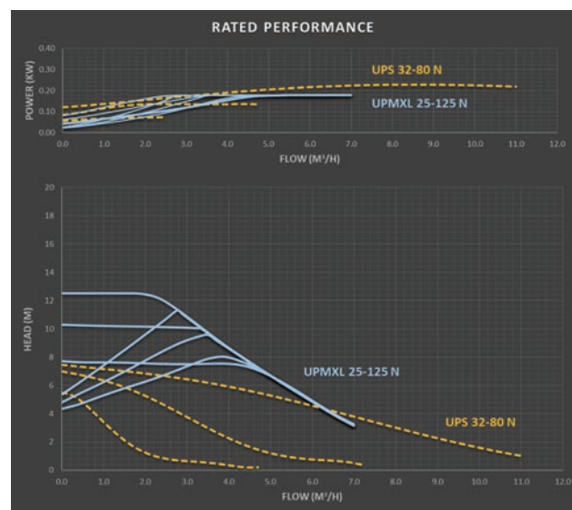
New UPM XL 25-125 and UPS 32-80 Secondary Pump Comparison Curves
